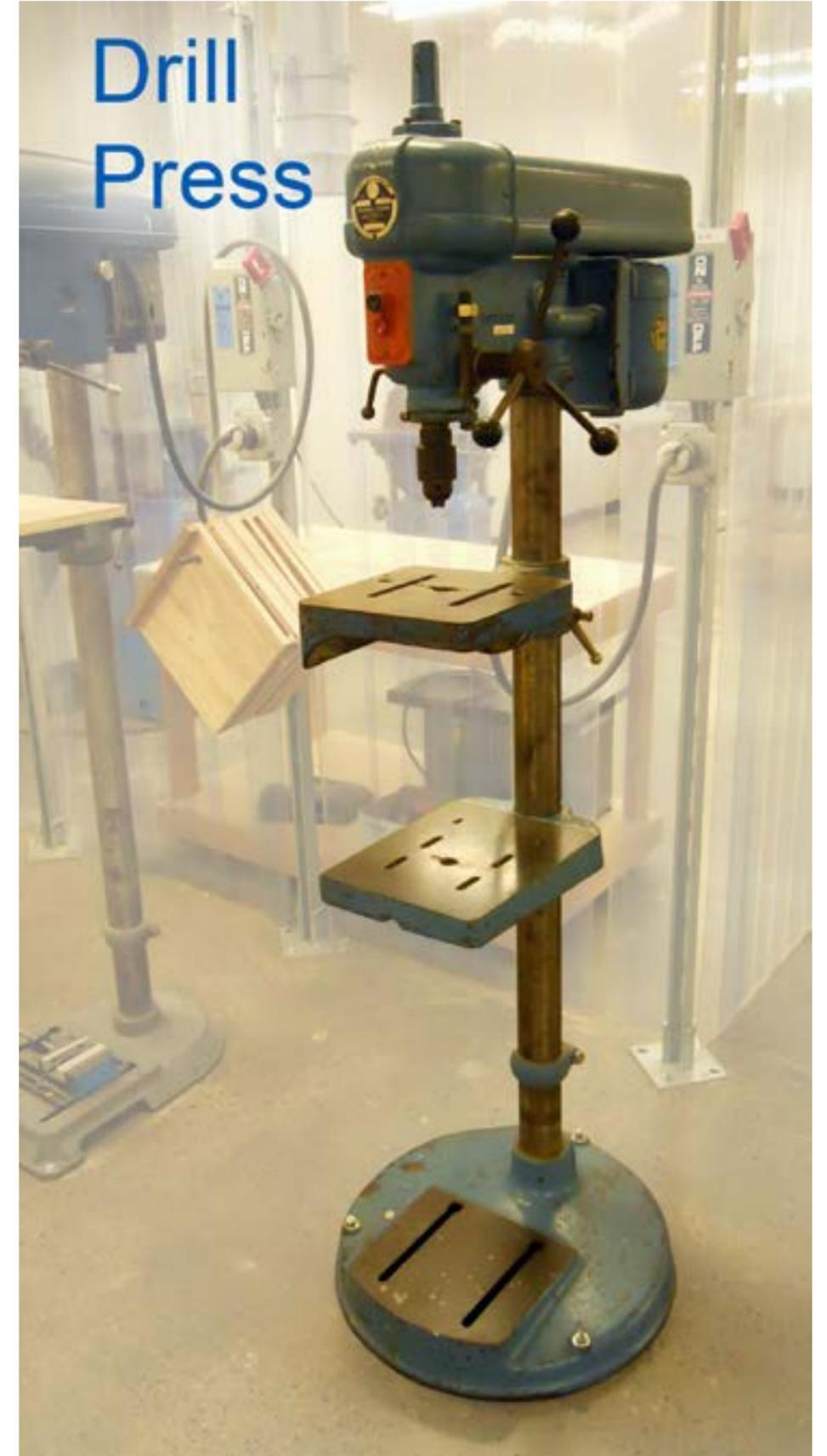
**Chuck-** A chuck is used to clamp and center a drill bit into a drill or drill press.
